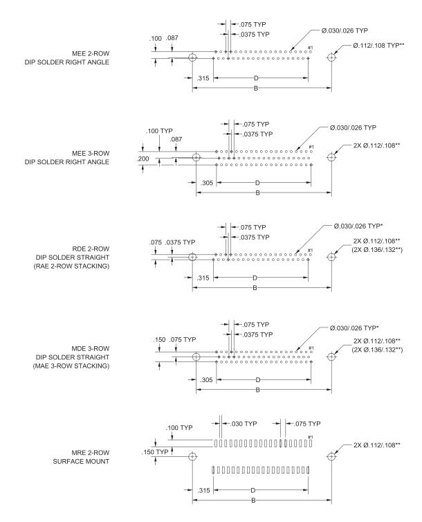
\*REQUIRED HOLE SIZE FOR COMPLIANT TERMINATION STYLE CONTACTS. FOR ALL OTHERS, HOLE SIZE SUBJECT TO USER MODIFICATION FOR APPLICATION OR ALTERNATIVE STANDARDS.
