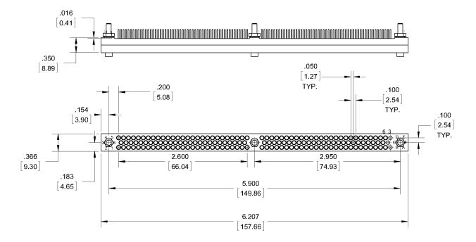
ONLY AVAILABLE WITH HARDWARE STYLE POLARIZED GUIDES WITH MOUNTING STUD (B)
